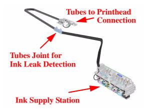
The Tubes move back and forth inside the volume defined by the Tube Guides. The Tube Guides are a pair of sheet metal parts with opposing U-shaped profiles.
