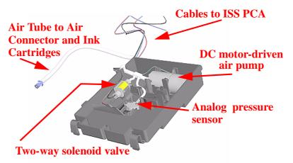
The APS pressurizes the ink in the Ink Cartridge bags by pressurizing the air around them. The Printer controls the air pressure using the pump with feedback from the sensor; when required the valve is opened to depressurize the air circuit. This allows control of the ink pressure at the inlet to the Printheads.
